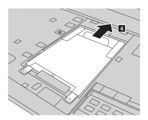
**7** Take out the hard disk drive secured in a metal frame **5**. **Lenovo IdeaPad Z380**
